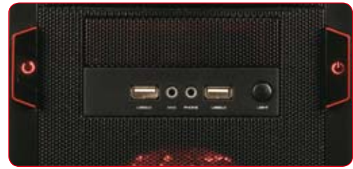
2x USB 2.0, HD/AC'97 Audio, button to select one of two fascinating Apollish light effects
